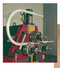
Aluminium profile bending with machine DELTA 50 CNC-C
