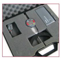
A specific wireless interface (optional) allows you to get and automatically send to the CNC-C the radius up to 25 m. long. This allows the creation and automatic editing of bending radius and any other kind of control.
