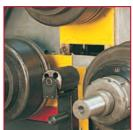
The machine performs all the operations necessary to complete desired sharpe until the bent profile comes out from the bending machine.
